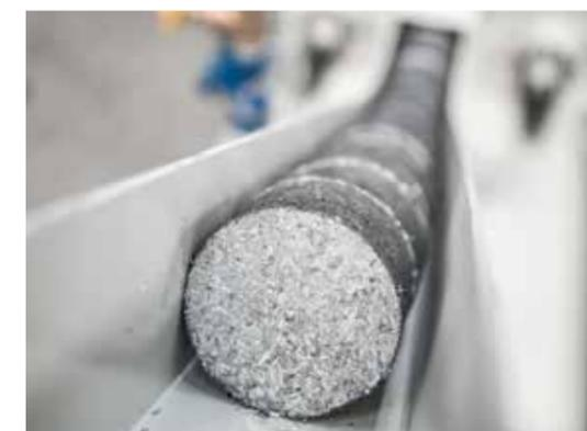
**Fitted with an automatic briquette length adjustment as standard**
